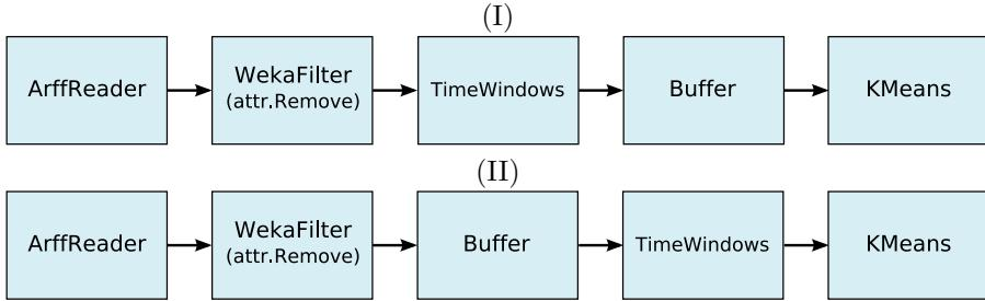
FIGURE 6: DPN of the first (batch) and second (stream) variant of experiment
