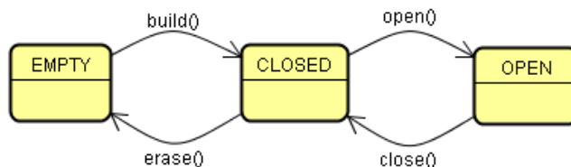
FIGURE 2: Diagram of cell states and allowed transitions
