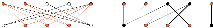
Figure 1. Left: sample bipartite graph G with a largest bipartite clique (colored vertices). Right: bipartite graph G' (complement of graph G ) with a largest matching (thick edges), a minimal vertex cover (black vertices) and a largest independent set (colored vertices).
