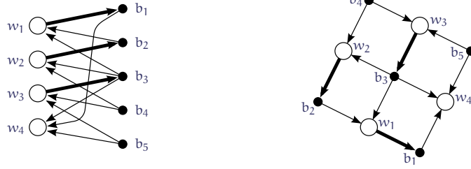
Figure 1.2: A matching-directed bipartite graph: matched edges are directed left-to-right, while unmatched edges are directed right-to-left. The M -alternating paths in G are exactly the directed paths of G^{\times M} .
