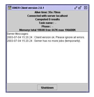
Figure 5.2: The DIXER Client connected to the DIXER Server. The Server currently has no jobs for this computer.
