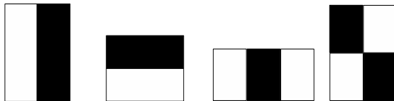
Fig. 1. Types of regions used in weak classifiers. White indicates positive sub-region and black negative sub-region
