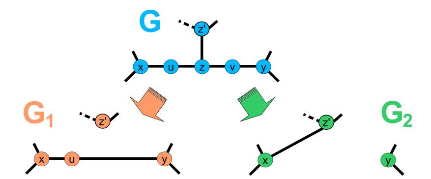
*G* is 3-edge-colorable iff  $G_1$  or  $G_2$  is 3-edge-colorable. How expensive is it? T(n) = T(n-2) + T(n-3) + poly(n), so  $T(n) = O(1.325^n)$
