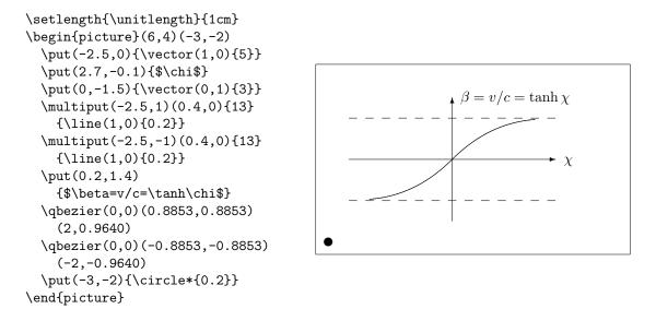
The control points of the two Bézier curves were calculated with formulas (5.1). The positive branch is determined by  $P_1 = (0, 0), m_1 = 1$  and  $P_2 = (2, \tanh 2), m_2 = 1/\cosh^2 2$ . Again, the picture is defined in mathematically convenient coordinates, and the lower left corner is assigned the mathematical coordinates (-3, -2) (black disk).
