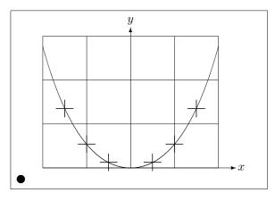
In this figure, each symmetric half of the catenary  $y = \cosh x - 1$  is approximated by a quadratic Bézier curve. The right half of the curve ends in the point (2, 2.7622), the slope there having the value m = 3.6269. Using again equation (5.1), we can calculate the intermediate control points. They turn out to be (1.2384, 0) and (-1.2384, 0). The crosses indicate points of the *real* catenary. The error is barely noticeable, being less than one percent.
