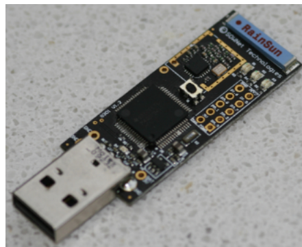
Fig. 1. G-Node G301 (housing disassembled)
