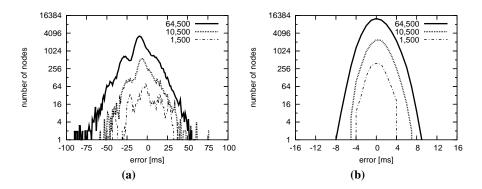
**Fig. 4.** Time accuracy of GTP: (a) using hop counts and sample filtering; (b) using the dispersion metric. Note the log scale for the y-axis and different scales for the x-axis.
