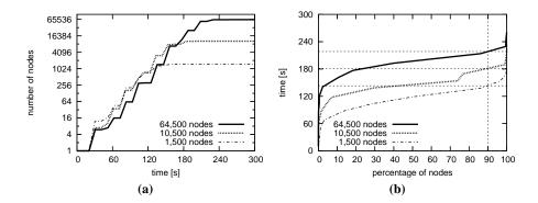
**Fig. 3.** Time dissemination speed of GTP: (**a**) shows that the number of nodes to which the time has been disseminated grows exponentially with time (note the log scale for the y-axis); the horizontal lines in (**b**), which approximate 90% dissemination, show that the dissemination time grows logarithmically with the size of the network.
