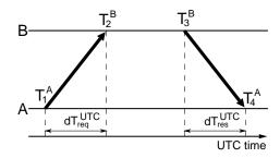
Fig. 1. Comparing time displayed by network clocks.
